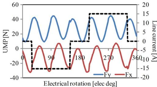
Fig. 6. UMP in the 25-slot stator machine when fully loaded with the force broken down into  $F_x$  and  $F_y$ —this shows a rotating force vector and a constant pull.
