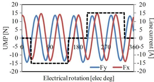
Fig. 5. UMP in the 25-slot stator machine when open circuit with the force broken down into  $F_x$  and  $F_y$ —this shows a rotating force vector.
