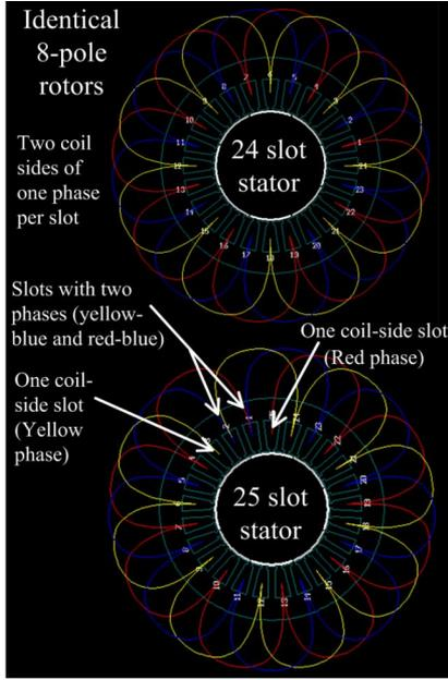
Fig. 1. The 24- and 25-slot three-phase windings.
