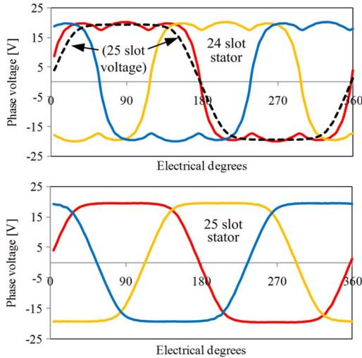
Fig. 2. The 24- (top) and 25- (bottom) slot stator machine open-circuit voltage at 1000 r/min. The 25-slot red phase is shown in the top graph for comparison.
