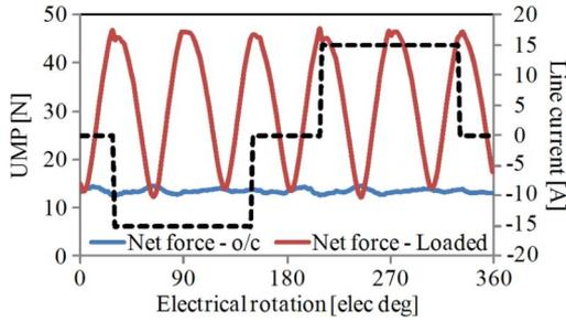
Fig. 4. UMP in a 25-slot stator machine when the machine is open circuit and fully loaded—radial force magnitude (which will vary in direction). The current waveform for phase 1 is given for reference.
