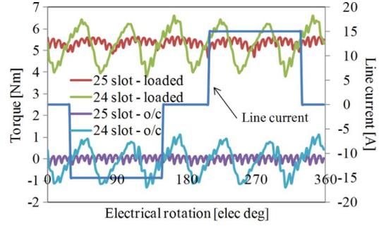
Fig. 3. The 24- and 25-slot stator machine—open-circuit cogging torque and load torque (the load current is 15 A peak and shown).
