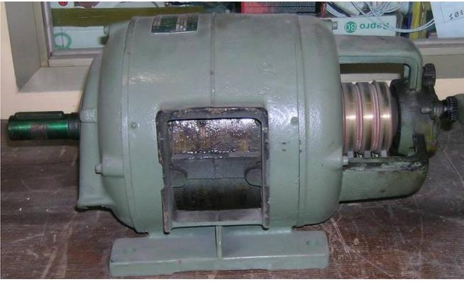
Fig. 5: WRIM under test.
