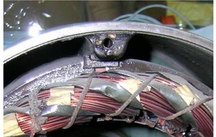
Fig. 6: One of the twelve stator core supports of the stator core.
