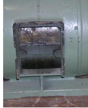
Fig. 8: Opening for the air speed measurement.
