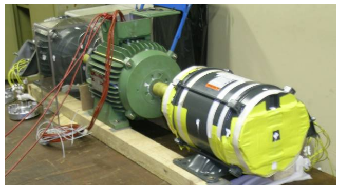
Fig. 4: Test bench with the two motors under test (Motor B in TEFC configuration)
