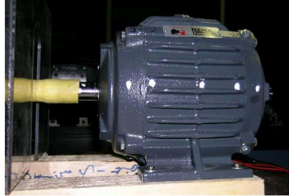
Fig. 1: Motor A (2 poles TEFC machine).
