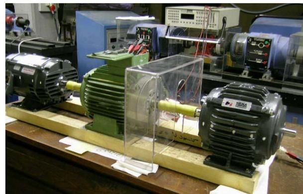
Fig. 4: Test bench with the two motors under test.
