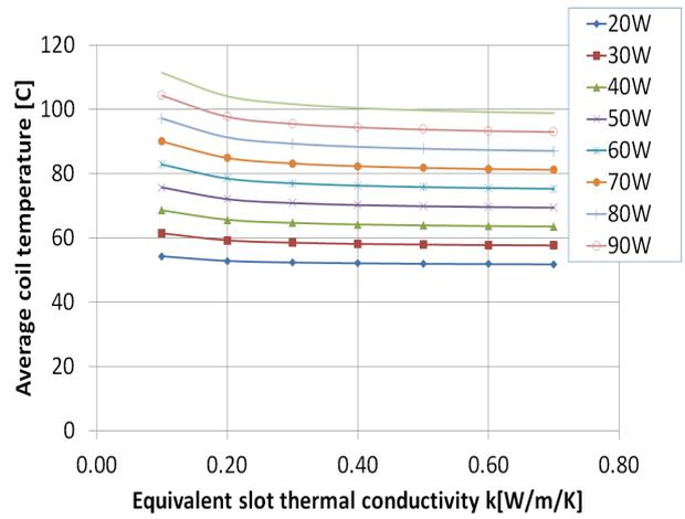
Fig. 14. Average coil temperature [ $^{\circ}\text{C}$ ] variation with equivalent thermal conductivity ( $k$  [ $\text{W}/\text{m}/\text{K}$ ]) and total copper loss [ $\text{W}$ ]; heat transfer coefficient is assumed to be  $55 \text{ W}/\text{m}^2/^{\circ}\text{C}$ .
