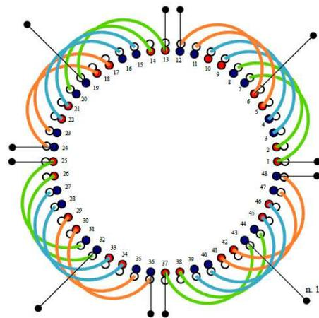
Fig. 17. Thermal sensors placement in the winding; 1<sup>st</sup> sensor is connected to the conductors in slot 48, 12<sup>th</sup> sensor is connected to the conductors in slot 43.
