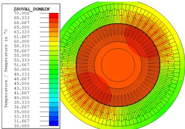
Fig. 13. Temperature isovalues distribution for the duplex 3-phase IM under faulty operation conditions (Fig. 2(c)).
