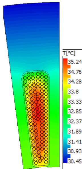
Fig. 5. Temperature distribution within the slot. Normal conditions, only copper losses are considered.
