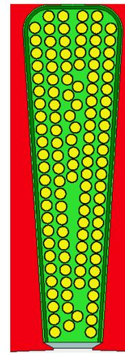
Fig. 4. Conductors random distribution in the slot
