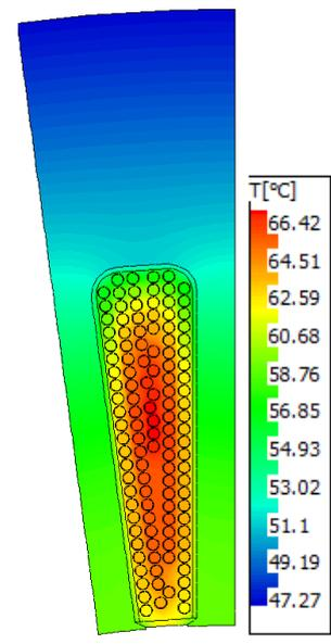
Fig. 6. Temperature distribution within the slot. Faulty conditions, only copper losses are considered.
