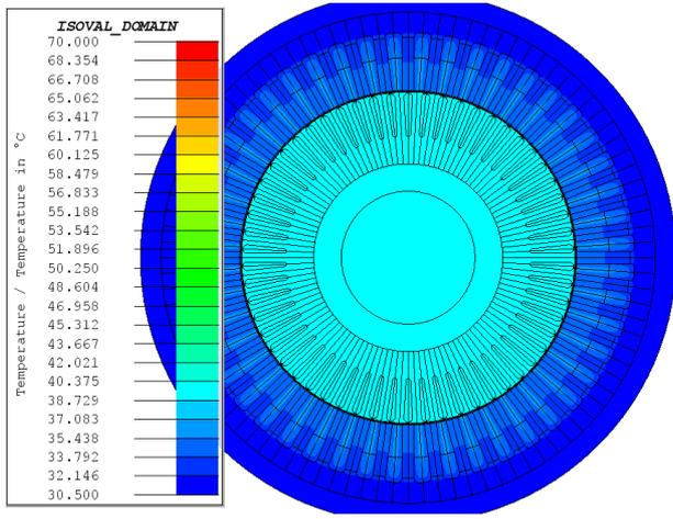
Fig. 11. Temperature isovalues distribution for the duplex 3-phase IM under normal operation conditions.
