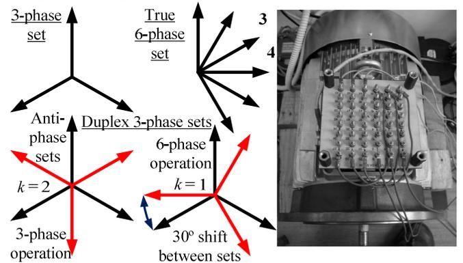
Fig. 1. Phase arrangements and terminal board of tested duplex 3-phase induction machine prototype.
