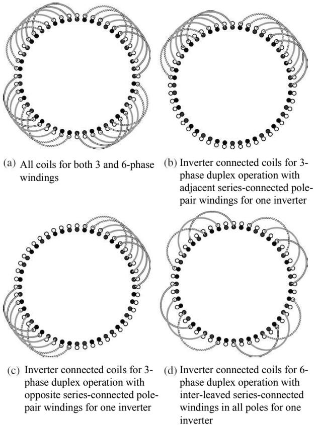
Fig. 2. Different winding configurations for the duplex connections – (a) all coils in machine; (b)-(d) coils for just one of the inverters.
