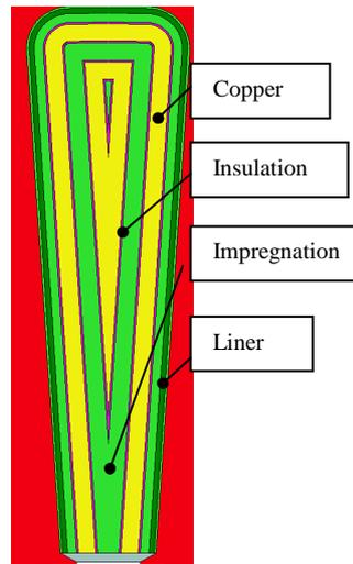
Fig. 3. Conductors layered model of the slot
