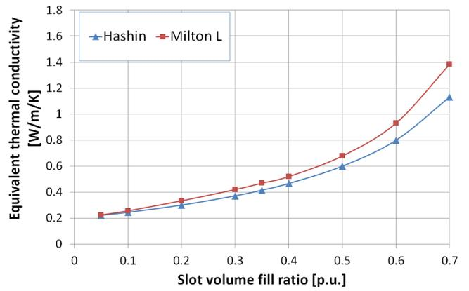
Fig. 10. Slot equivalent thermal conductivity variation with slot volume fill ratio.
