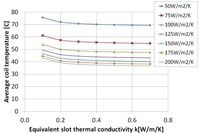
Fig. 16. Average coil temperature [ $^{\circ}\text{C}$ ] variation with equivalent thermal conductivity ( $k$  [ $\text{W}/\text{m}/\text{K}$ ]) and equivalent heat transfer coefficient ( $HTC$  [ $\text{W}/\text{m}^2/\text{K}$ ]); total copper loss is assumed to be  $100 \text{ W}$ .
