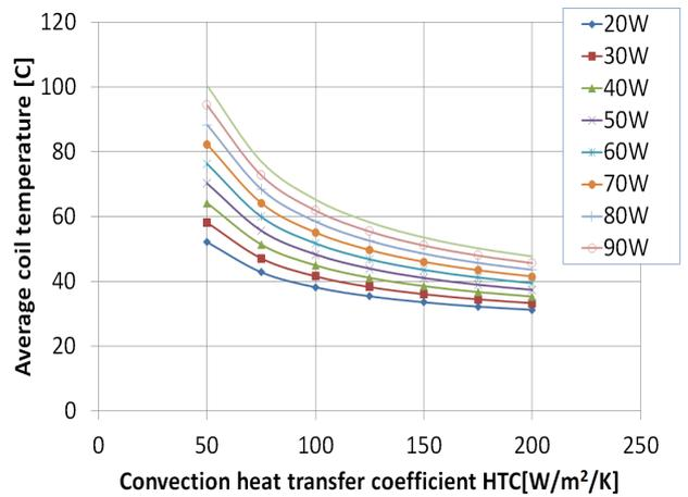
Fig. 15. Average coil temperature [ $^{\circ}\text{C}$ ] variation with equivalent heat transfer coefficient ( $HTC$  [ $\text{W}/\text{m}^2/\text{K}$ ]) and total copper loss [ $\text{W}$ ]; equivalent slot thermal conductivity is assumed to be  $0.5 \text{ W}/\text{m}/\text{K}$ .
