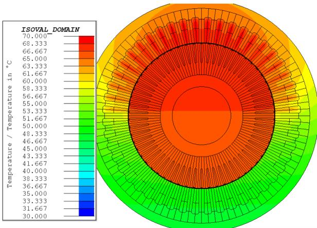
Fig. 12. Temperature isovalues distribution for the duplex 3-phase IM under faulty operation conditions (Fig. 2(b)).
