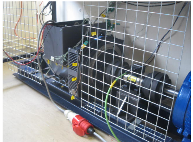
Figure 10: Alternator thermal analysis test-rig set-up.
