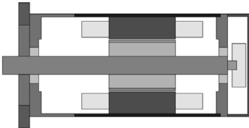
Fig. 2. Axial section in MotorCAD
