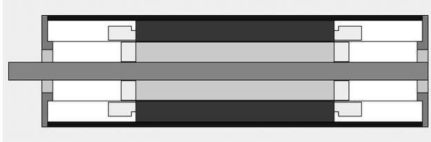
Fig. 6. MotorCAD axial section for induction motor
