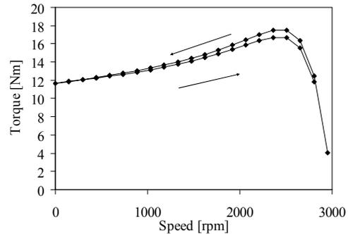
Fig. 21. Torque/speed curve over 5 second test at 400 V
