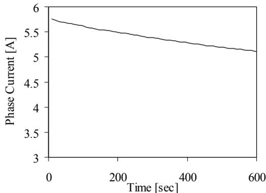
Fig. 14. Phase current variation over 10 minutes at 400 V and 2886 rpm
