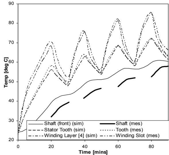
Fig. 4. Comparison between measured and simulated temperatures in the brushless permanent machine
