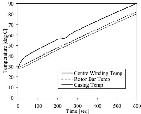
Fig. 13. Temperature variation over 10 minutes at 400 V and 2886 rpm
