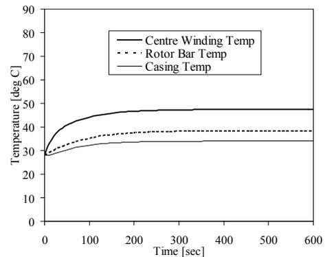
Fig. 16. Temperature variation over 10 minutes at 400 V and 2886 rpm with external casing water cooling
