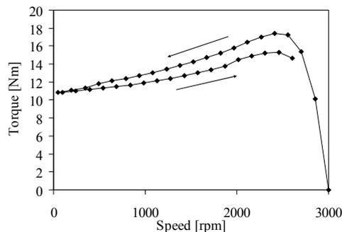
Fig. 18. Torque/speed curve over 20 second test at 400 V
