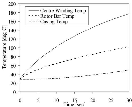
Fig. 10. Temperature simulations at locked rotor and rated 400 V
