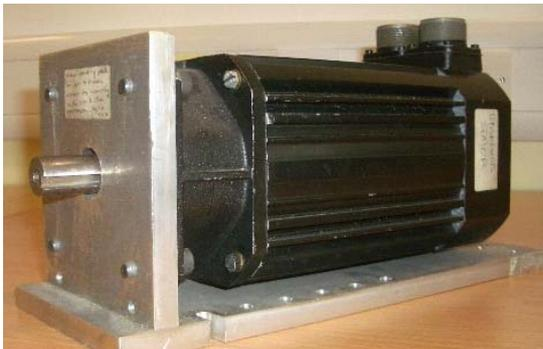
Fig. 3. Actual brushless permanent magnet motor
