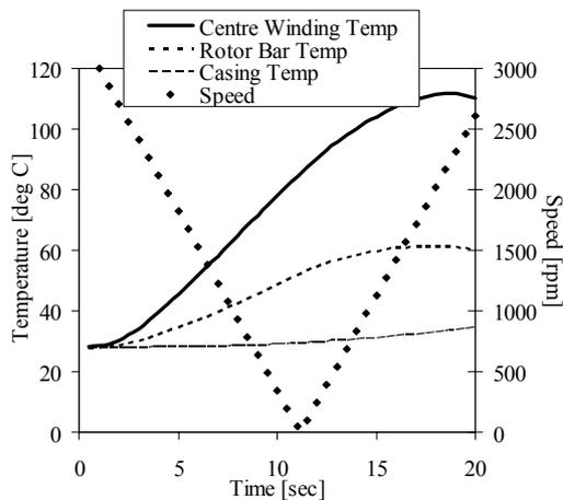
Fig. 17. Variation of temperature with time for a torque/speed curve at 400 V
