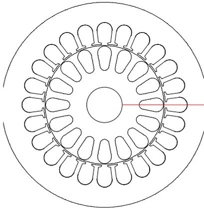
Fig. 5. PC-IMD cross section for induction motor
