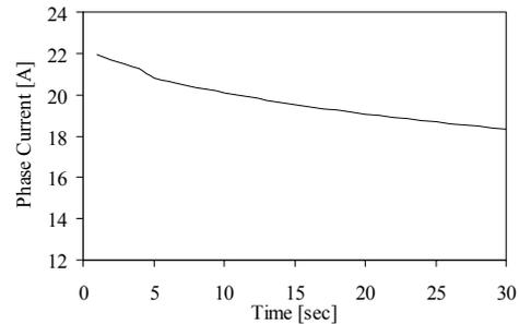
Fig. 11. Phase current prediction at locked rotor and rated 400 V
