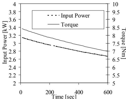
Fig. 15. Input power and torque over 10 minute at 400 V and 2886 rpm
