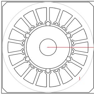
Fig. 1. Brushless permanent magnet motor cross section in PC-BDC
