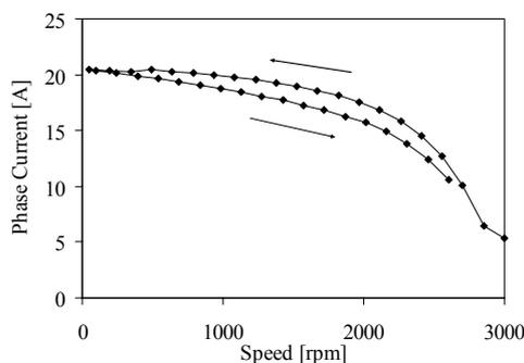
Fig. 19. Current/speed curve over 20 second test at 400 V
