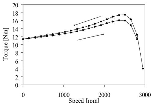
Fig. 20. Torque/speed curve over 10 second test at 400 V
