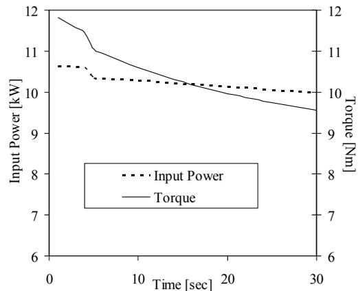
Fig. 12. Input power and torque predictions at locked rotor and rated 400 V
