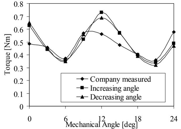
Fig. 7. Variation of locked rotor torque at 90 V and ambient temperature
