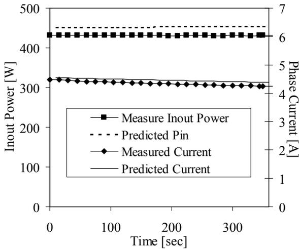
Fig. 9. Comparison between the measured and predicted input power and phase currents at 90 V
