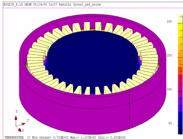
Fig 10: FEM computation of temperature distribution.
