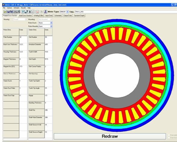
Fig 1: Radial section description of the machine.
