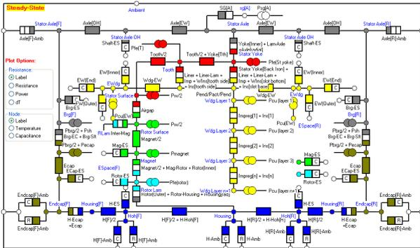
Fig 7: Thermal schematic solved
