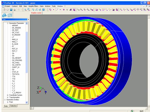
Fig 8: Geometry description by FEM software
