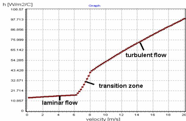
Fig 8: Enclosed channel forced convection
