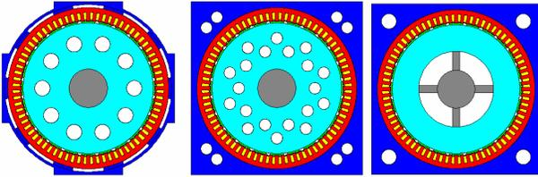
Fig 10: Examples of typical through ventilation duct types
