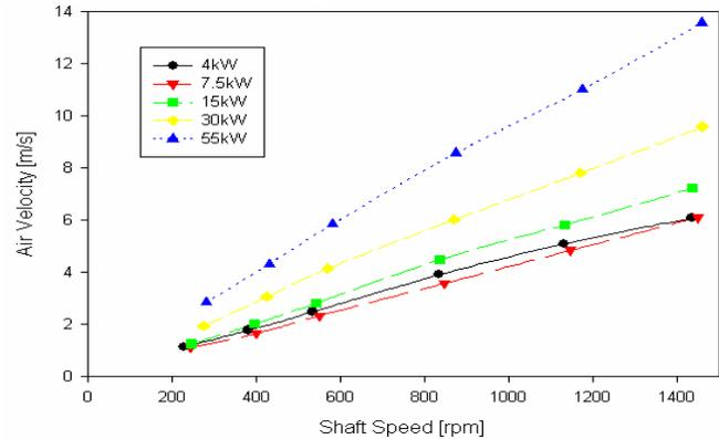
Fig. 5: Variation in fin channel air velocity with RPM (motors in Fig 3)
