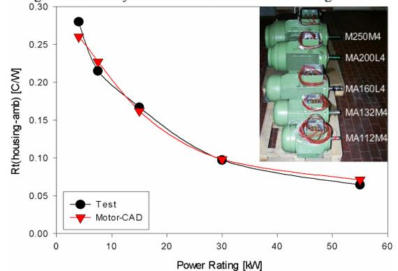
Fig. 3: Natural convection resistance - housing to ambient
