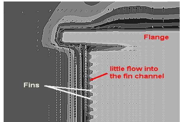
Fig 2: CFD Analysis – radial fins with vertical flange mount
