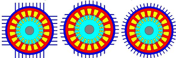
Fig 4: Examples of housing types suitable for TEFC cooling
