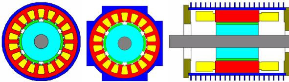
Fig 1: Examples of housing types suitable for TENV cooling
