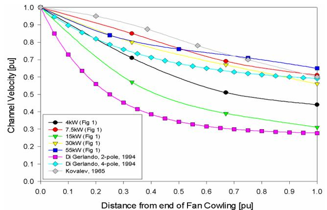
Fig. 6: Fin channel air velocity reduction with distance from fan
