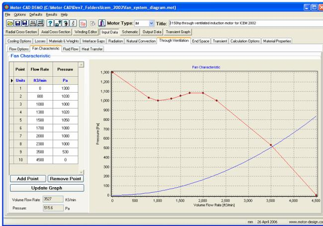
Fig 11: Fan and system resistance characteristics
