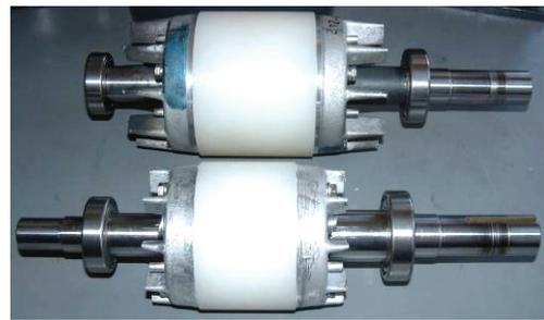
Fig.1: Prototype plastic rotors
