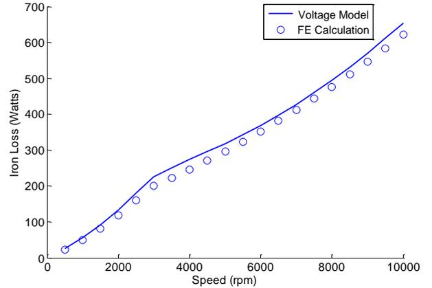
Figure 8: Comparison of voltage model with FE calculations
