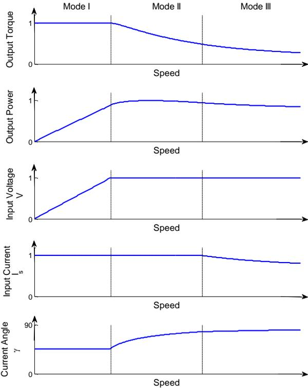
Figure 2: Field weakening behaviour of a BLAC PM motor [7]
