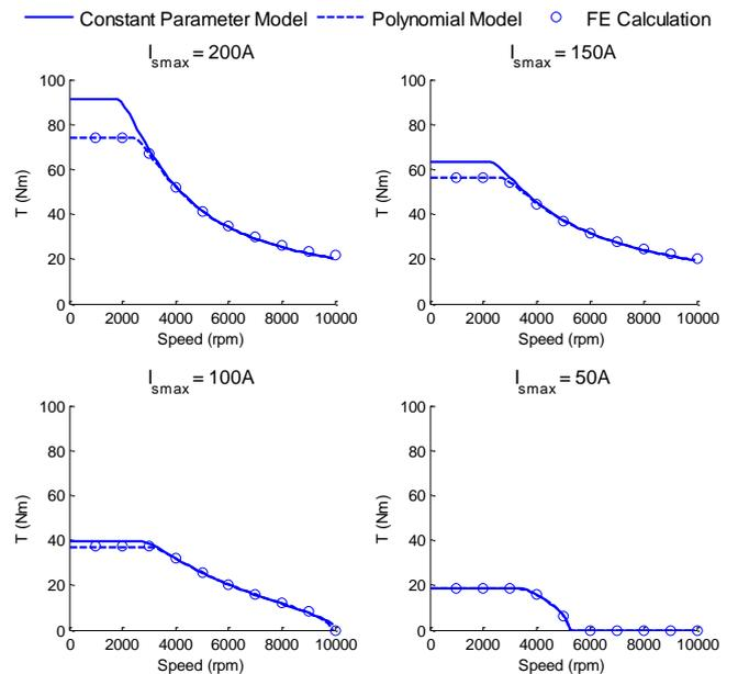
Figure 7: Comparison of torque/speed plots calculated using the constant parameter and flux linkage model
