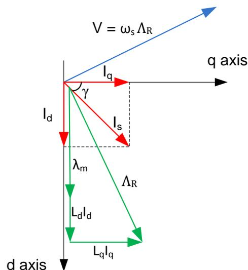
Figure 1: Phasor diagram for a salient PM BLAC motor
