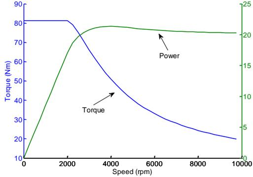
Figure 3: Calculated torque and power speed characteristics
