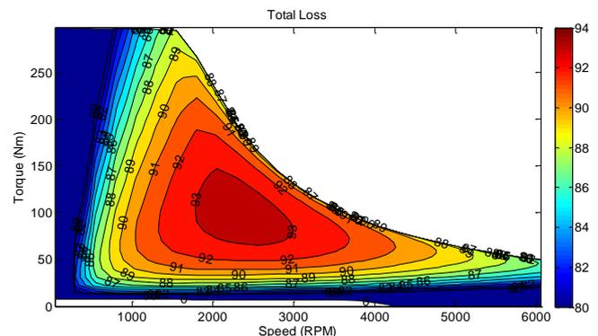
Figure 10: Computed Efficiency Map for 2004 Toyota Prius Motor
