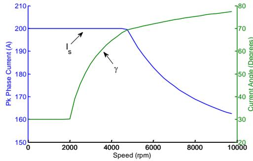
Figure 4: Calculated optimum  $I_s$  and  $\gamma$  with increasing speed
