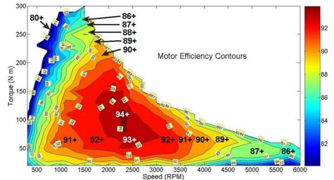
Figure 9: Measured Efficiency Map for 2004 Toyota Prius Motor [1]
