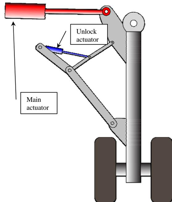
Fig.1. Schematic of undercarriage, showing actuators
