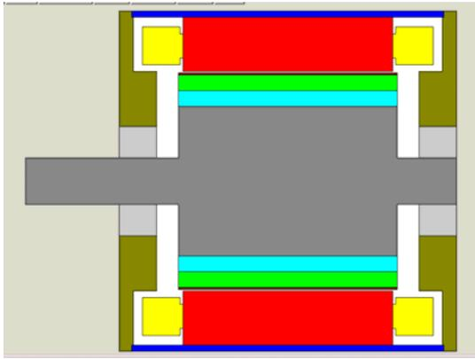
Fig.5. Motor-CAD axial cross-section
