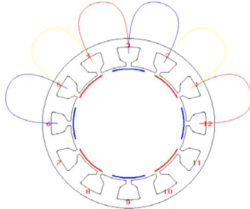
Fig.3. Insertion pattern for one winding
