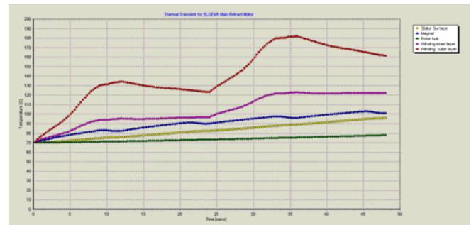
Fig.8. Temperature vs. time starting from  $70^{\circ}\text{C}$  ambient
