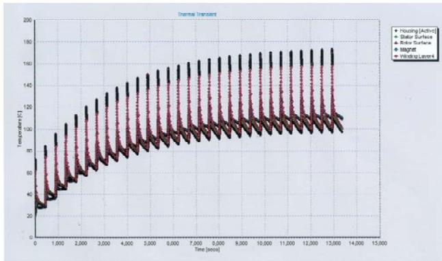
Fig.9. Temperatures resulting from many repetitions of a reduced duty cycle
