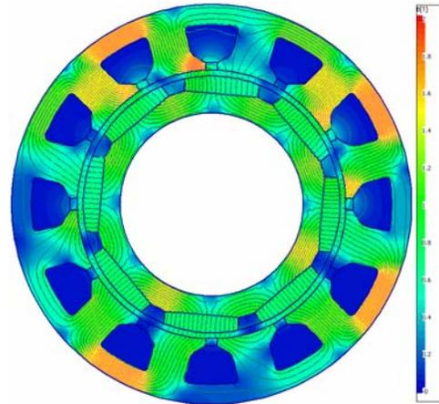
Fig.4. Flux distribution under full-load
